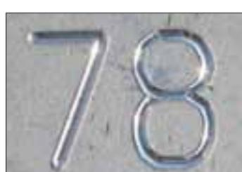
**Vibrating pin** - Characters marked with small pin vibration. Recommended for speed marking with a very high quality.
