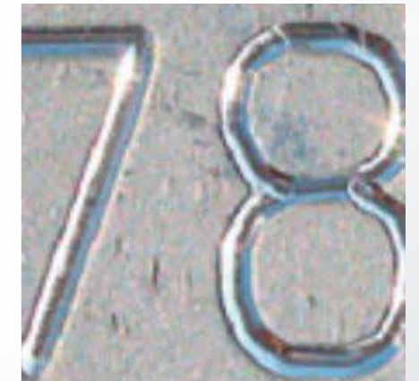
SCRIBE MARKING Markings are made by striking the surface and removing the material for deep and silent marking.
