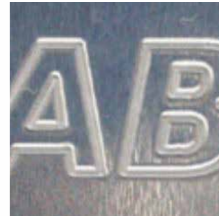
VIBRATING DOT PEEN Characters are marked with a small pin while vibrating. Highly recommended for fast marking with very high quality needs.
