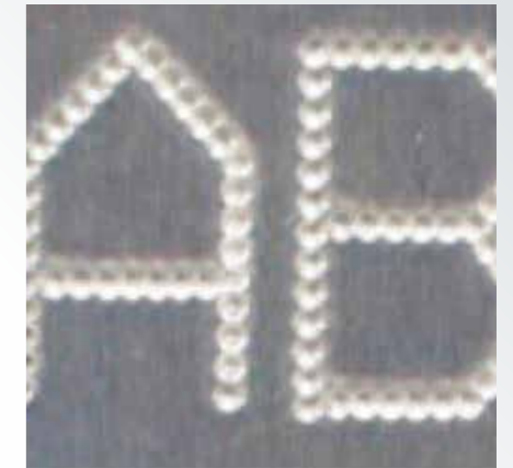
PNEUMATIC DOT PEEN The Pin is moved automatically by opening and closing the drive and return air. Recommended for marking on irregular and rough surfaces.
